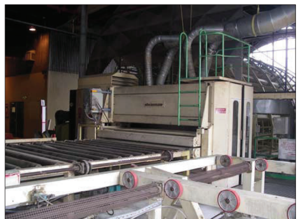
A Typical High Speed Automated Sander
